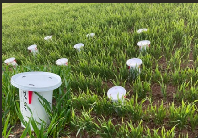
Figure 2: Setup for ammonia measurement in the field.
